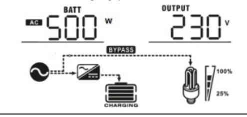
Battery voltage and output voltage
