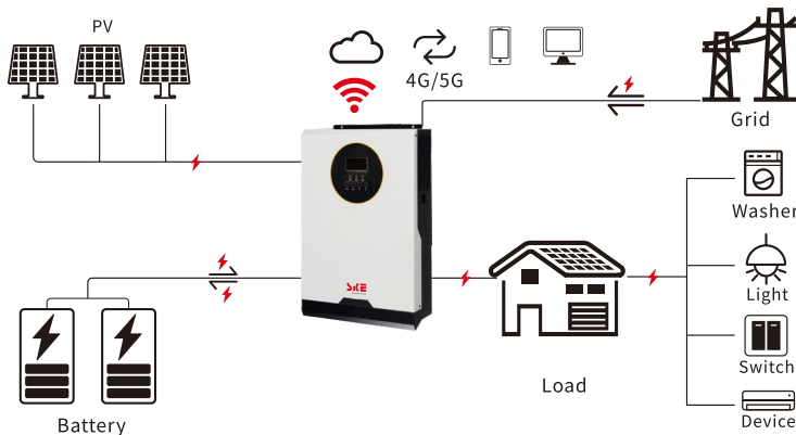
Home energy storage system
